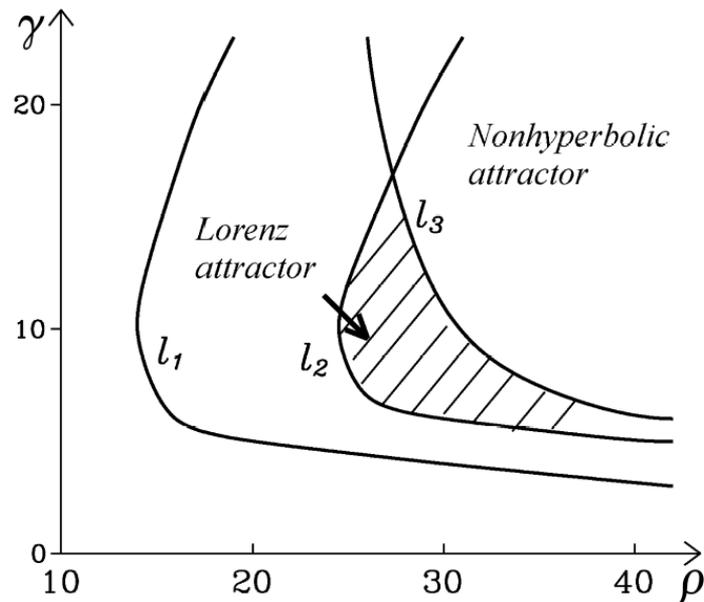
Bifurcation diagram of the Lorenz system (3) on the  $(\rho, \gamma)$  parameter plane for  $b = 8/3$ . The transition from the Lorenz attractor to a non-hyperbolic attractor is observed when one intersects the line  $l_3$ .
