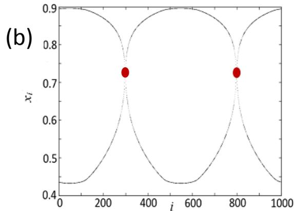
Snapshot (a) and space-time profile (b) for  $\sigma = 0.43$  (2-periodic oscillation regime in the ring elements)
