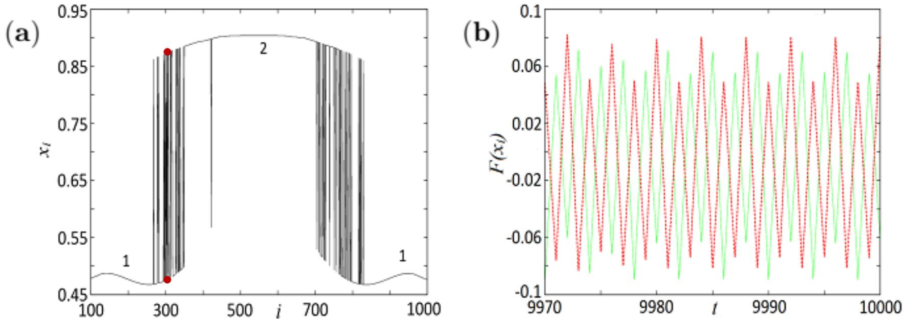
Snapshot (a) of the dynamics of the coupled logistic maps (1) and time series of the coupling function  $F(x_i)$  for the 318th element (solid green line) and the 319th element (dotted red line) of the ring (b). The coupling strength is chosen as  $\sigma = 0.27$ .
