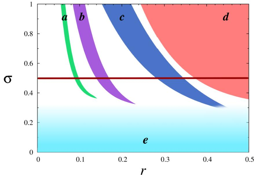
Regions of coherence for non-locally coupled Henon maps (1) in the  $(r, \sigma)$  parameter plane with wave numbers  $k = 1, 2$  and 3 (regions **(c)**, **(b)** and **(a)**, respectively). **(d)** is the area of completely synchronized chaotic states, **(e)** is the region of complete incoherent states. Chimera states are observed for  $\sigma < 0.5$ . Parameters:  $\alpha = 1.4$ ,  $\beta = 0.3$ ,  $N = 1000$ .
