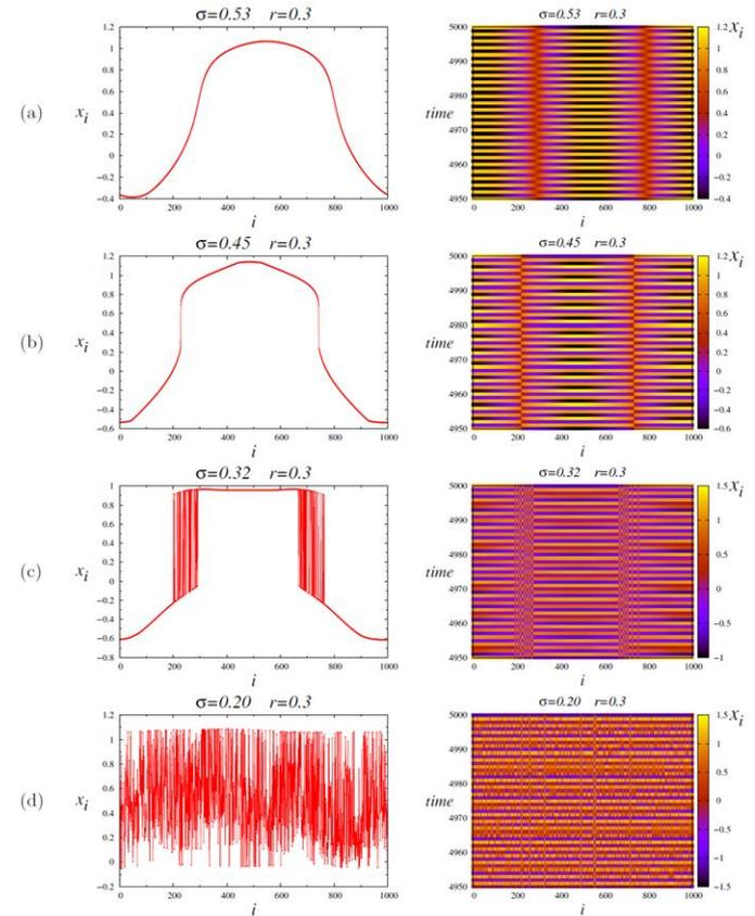
Coherence-incoherence bifurcation for coupled Henon maps with fixed coupling radius  $r = 0.3$ . For each value of the coupling parameter (decreasing from top to bottom,  $\sigma = 0.53$ ,  $\sigma = 0.45$ ,  $\sigma = 0.32$  and  $\sigma = 0.2$ ), snapshots in time  $t = 5000$  (left columns) and space-time plots (right columns) are shown.
