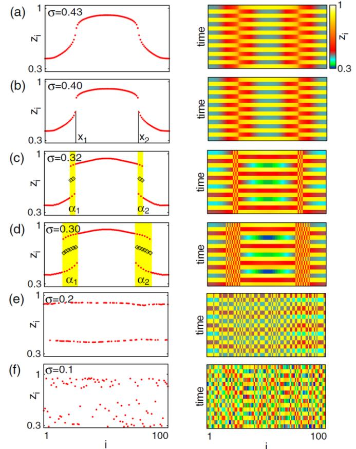
Coherence-incoherence bifurcation for coupled chaotic logistic maps for fixed coupling radius  $r=0.32$ . Snapshots (left columns) and space-time plots (right columns) for different values of coupling strength are shown.
