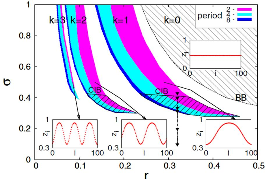
Regions of coherence for the system in the parameter plane  $(\sigma, r)$  with wave numbers  $k = 1, 2, \text{ and } 3$ . Snapshots of typical coherent states  $z_i$  are shown in the insets. The color code inside the regions distinguishes different time periods of the states.
