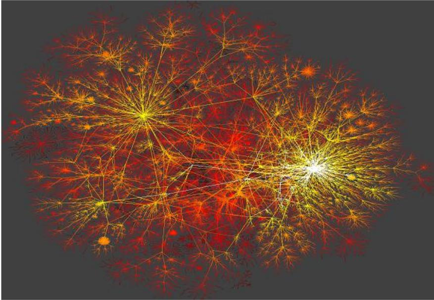
Traditionally the analysis of **the Internet structure** is made by means of ***traceroutes***. That is to say, by exploring all the paths from a given point to all the possible destinations.
