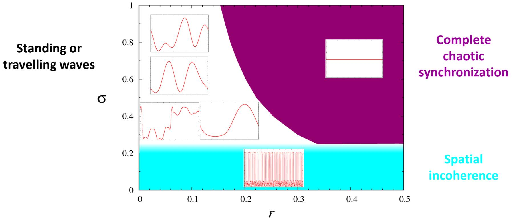
The structure of the parameter plane  $(r, \sigma)$  for the ring of non-locally coupled Lozi maps.
