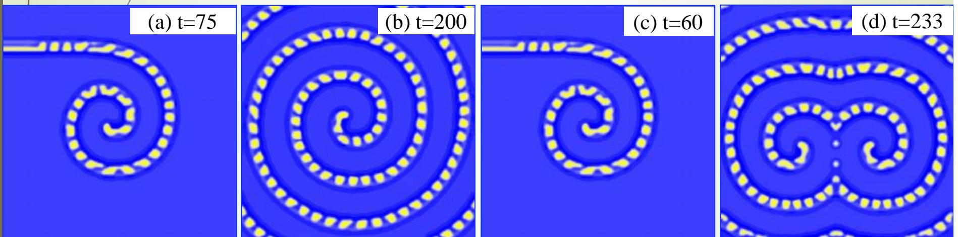
(a, b) Formation of a segmented spiral and (c, d) interaction of two segmented spirals in two-dimensional  $100 \times 100$  system with zero flux boundary conditions. Model parameters:  $\varepsilon=0.09$ ,  $\gamma_1=0.5$ ,  $\delta_1=0.7$ ,  $D_1=0.1$ ,  $\gamma_2=0.5$ ,  $\delta_2=0.5$ ,  $D_2=0.05$ ,  $\alpha=5$ ,  $I_c=0.1$ ,  $\Delta=0.03$ .
