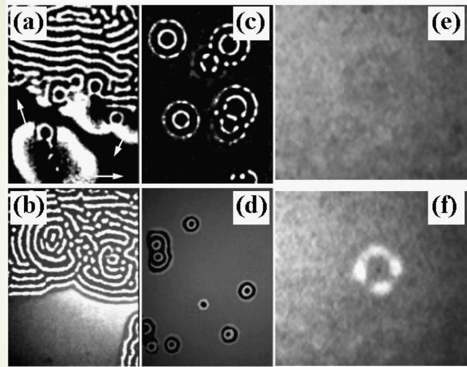
Turing patterns (a),(b), localized Turing patterns (c), and oscillons (d) –(f) in the Ru(bpy) - (a),(c),(e),(f ) and ferroin - (b),(d) catalyzed BZ-AOT systems.
