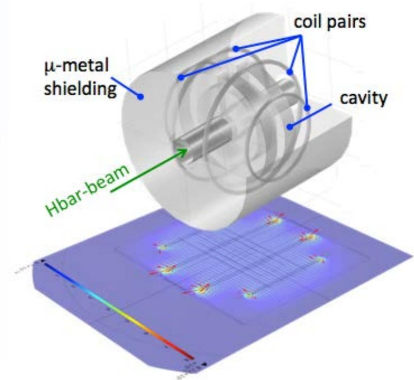
coils & shielding geometry optimized in COMSOL
