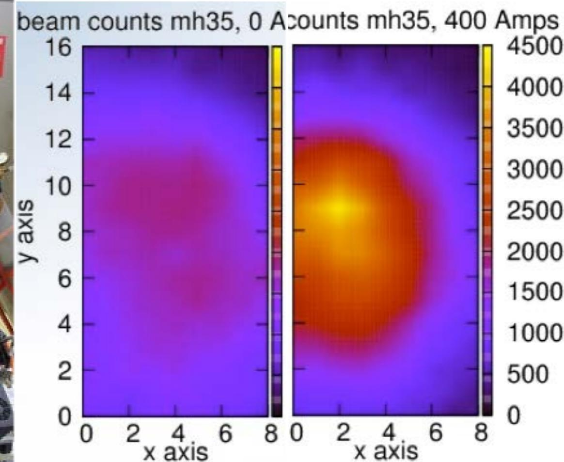
beam focusing by superconducting sextupole observed
